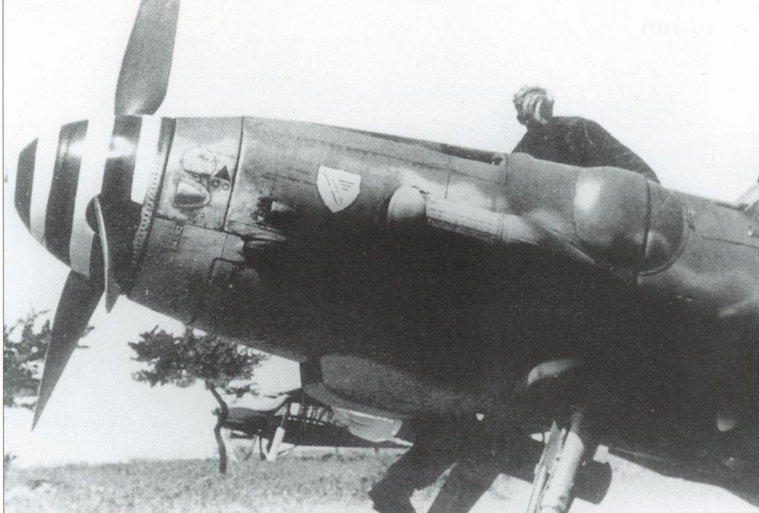
Above: A mechanic works on a Messerschmitt Bf 109G/R2 of Jagdgeschwader 3 'Udet', used on the Eastern Front for ground support tasks. The 'bump' on the forward fuselage houses the breech-block of a 13mm Maschinengewehr (MG) 131.
