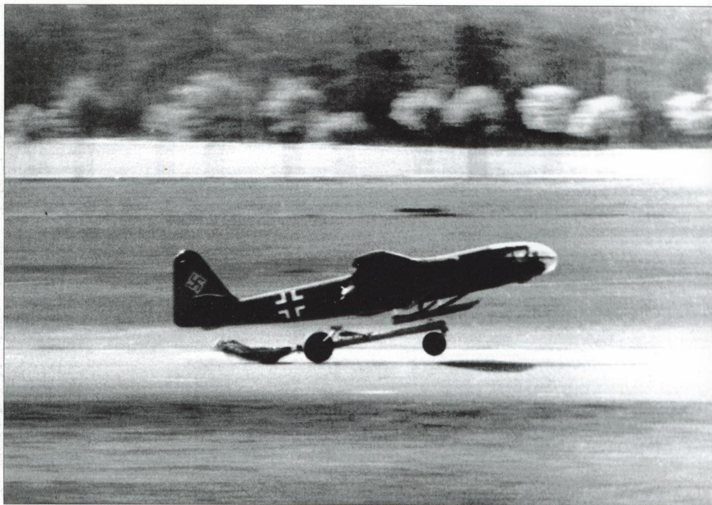
Above: One of the 'A' series prototypes of the Arado Ar 234 Blitz jet-powered bomber at the moment of take-off, April 1944. The undercarriage trolley has just been disengaged.
