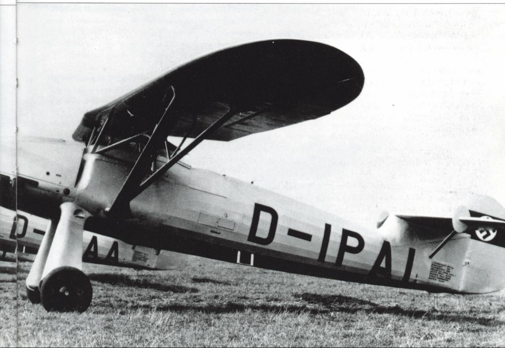
Below: Focke-Wulf Fw 56 Stösser fighters, 1936. An agile and clean-lined aircraft, the Fw 56 could be armed with one or two machine guns, and was used in early dive-bombing experiments.
