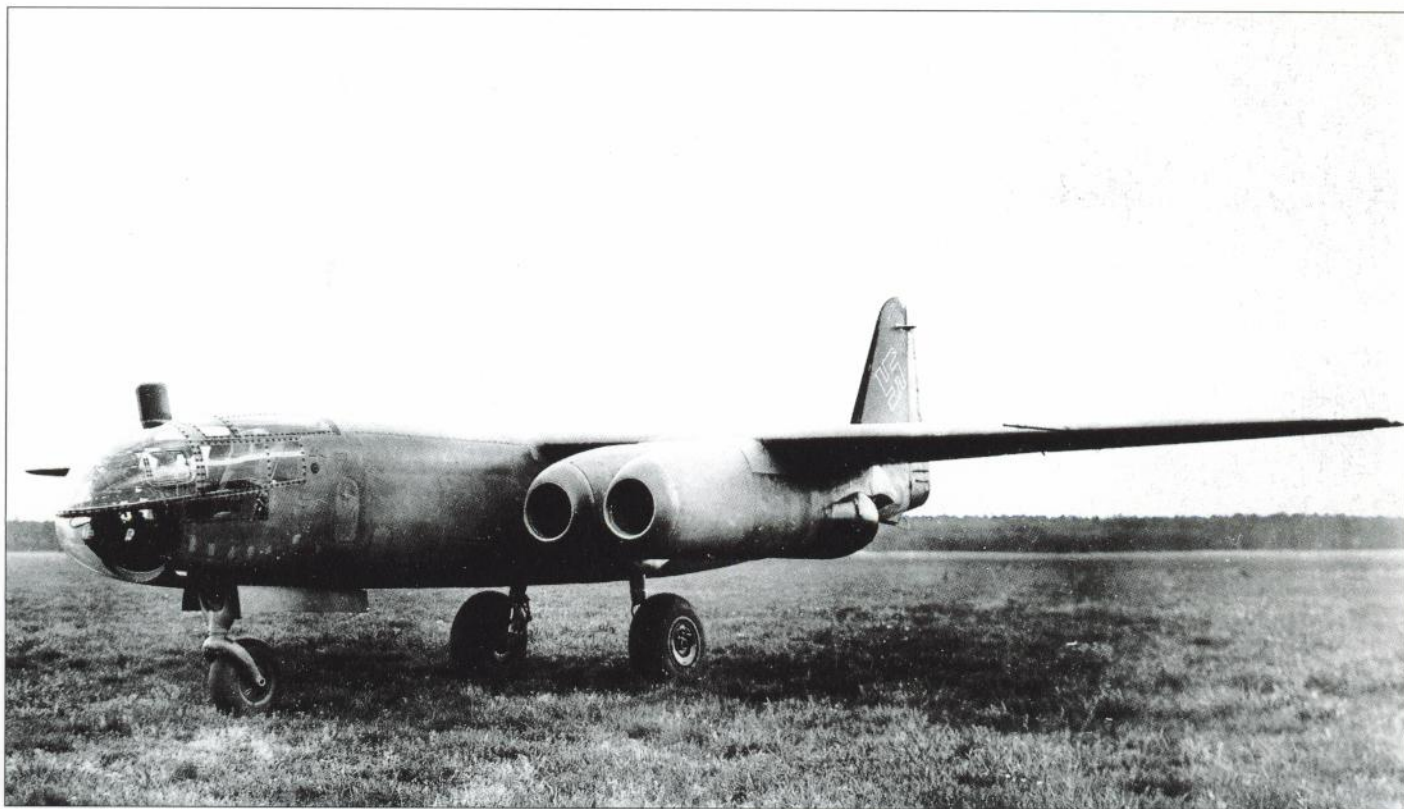
Above: The Ar 234 was the subject of a number of experiments during its short life-span. Here, the Ar 234 V13 variant mounts four BMW 003A-1 turbojets, mounted in pairs on each wing, in an effort to improve power and speed.
