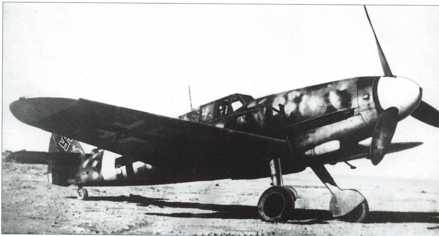
Above: A Messerschmitt Bf 109G fighter, characterised by its smooth cowling lines and enlarged under-nose air filter, stands on an airfield in Sicily, late 1942. The camouflage scheme breaks up the contours of the aircraft when viewed from the top or side.
